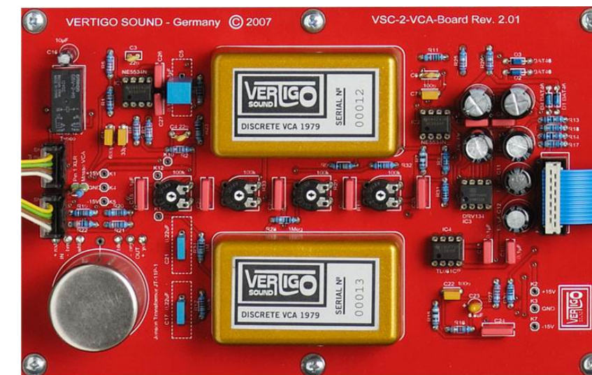
One (of two) VSC-2 boards hosting 2 of the 1979 VCAs each.
